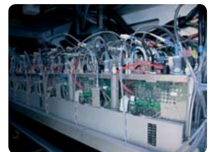
Print-head array: 24 print modules with 24 FUJIFILM Dimatix Spectra print heads per module
